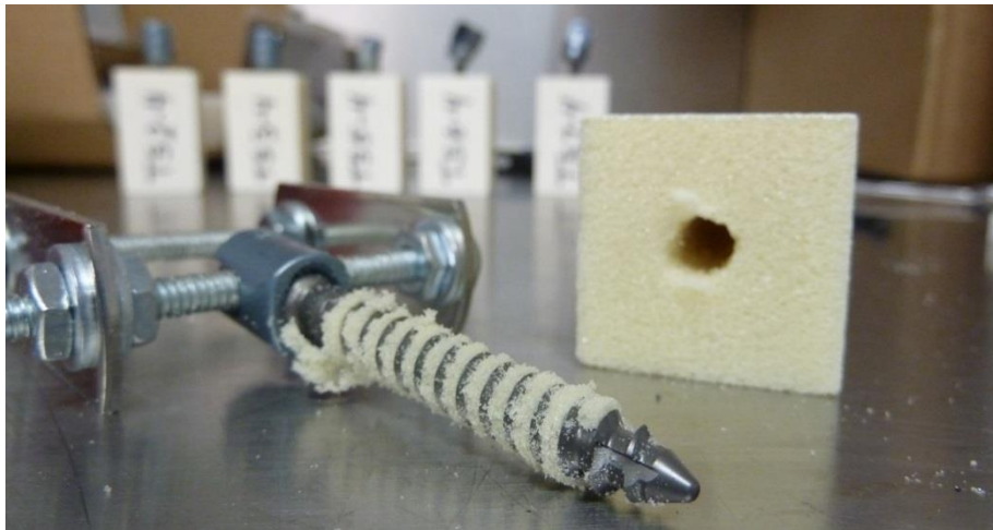
Figure 4.3. Standard screw damage to trabecular test block.
